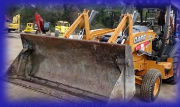
# 63609 2WD, STANDARD HOE, ROPS, AUX HYD, 4N1 BKT, WITH 1250 lb. Okada BREAKER $66,500
